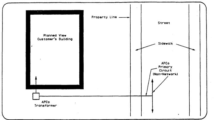
Designated Underground Area · Building Set Back From Property Line · Primary Underground to Transformer Located Outside of Building · Secondary Underground Service · Secondary Metering
