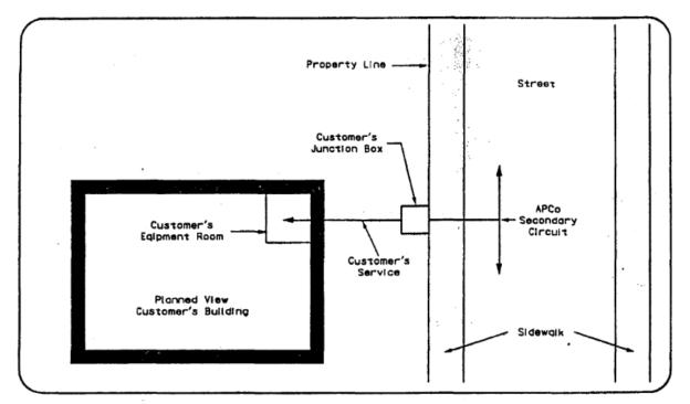
Designated Underground Area Building Set Back From Property Line Secondary Underground Service Secondary Metering
