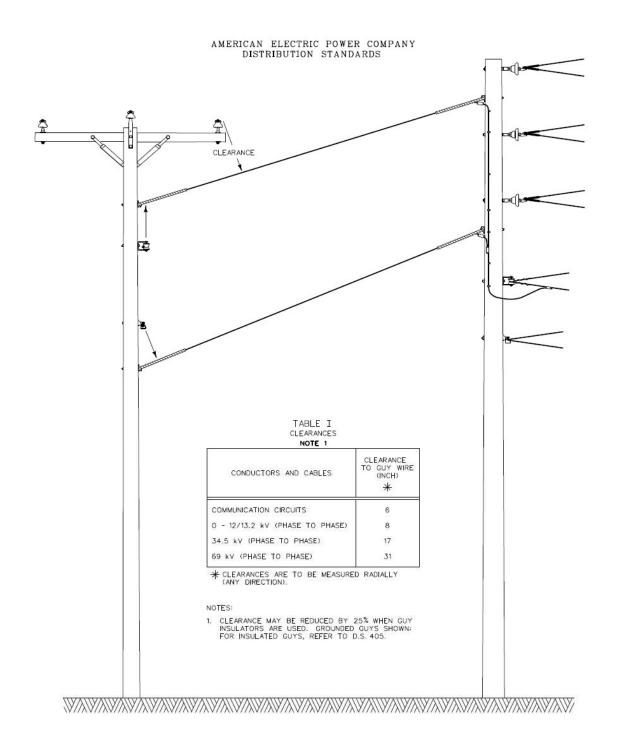
CLEARANCES BETWEEN SPAN GUYS AND LINE CONDUCTORS TRANSVERSE TO EACH OTHER ATTACHED TO SAME STRUCTURES
