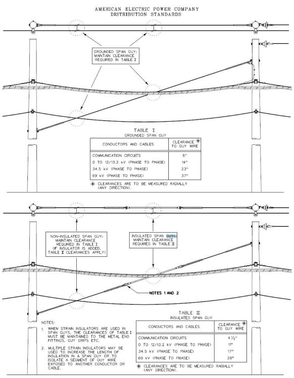
CLEARANCES BETWEEN SPAN GUYS AND LINE CONDUCTORS PARALLEL TO EACH OTHER ATTACHED TO THE SAME STRUCTURE
