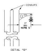
NON AEP COMMUNICATION CABLE ON MULTIPLE CONDUIT INSTALLATIONS
